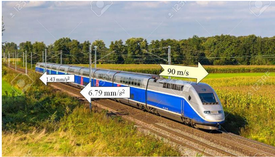
Figure 18: A TGV train is running on a straight rail from Rennes to Paris at 47-48° latitude. With a speed of u_r = 90 \text{ m/s} and at a distance from the Earth rotational axis of 4262 kilometers it is affected by two southward accelerations together 8.2 \text{ mm/s}^2 . One is due to the Coriolis effect ( 6.79 \text{ mm/s}^2 ) and the other to the curvature of the latitude ( 1.43 \text{ mm/s}^2 ). The latter acceleration, always directed towards the equator 6 , would be present also on a non-rotating Earth. If the train had run in the opposite direction, from east to west, the Coriolis force 2\Omega\sin(\text{latitude})u_r per mass unit would be directed in the opposite direction, towards the north and the total acceleration, now northward, would be 5.36 \text{ mm/s}^2 .
