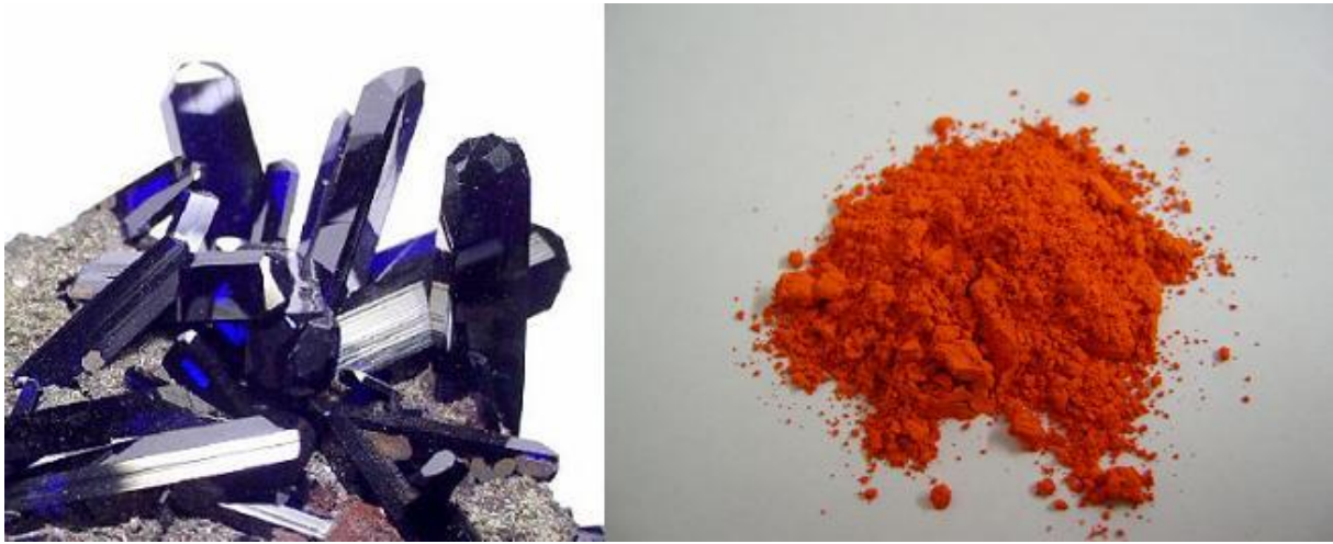
Figure 9: On the left, azurite ore; on the right, minium powder. Azurite (blue in colour) is a copper carbonate that has been known since Antiquity – traces of it have been found in Egyptian ointment pots. Minium is a lead tetroxide with the formula Pb_3O_4 , and has also long been used as a wall-painting pigment.
